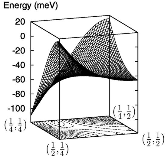
FIG. 4. Surface plot (and contour plot below) of the van Hove singularity in  $\epsilon_k$  (relative to  $E_F$ ) in the  $\Gamma$ - $M$ - $X$  plane, with  $M$  at the right-hand corner (planar coordinates are given in units of  $2\pi/a$ ). Note the extreme flatness of the dispersion along the diagonal  $M \rightarrow \Gamma$ . The negative effective mass sheet of the vHs lies in the third direction.
