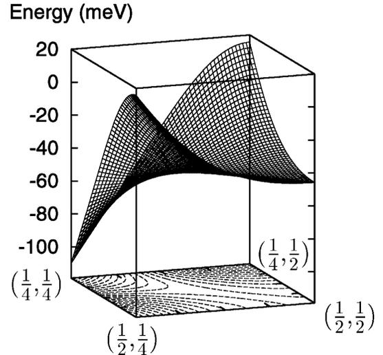
FIG. 4. Surface plot (and contour plot below) of the van Hove singularity in  $\epsilon_k$  (relative to  $E_F$ ) in the  $\Gamma$ - $M$ - $X$  plane, with  $M$  at the right-hand corner (planar coordinates are given in units of  $2\pi/a$ ). Note the extreme flatness of the dispersion along the diagonal  $M \rightarrow \Gamma$ . The negative effective mass sheet of the vHs lies in the third direction.
