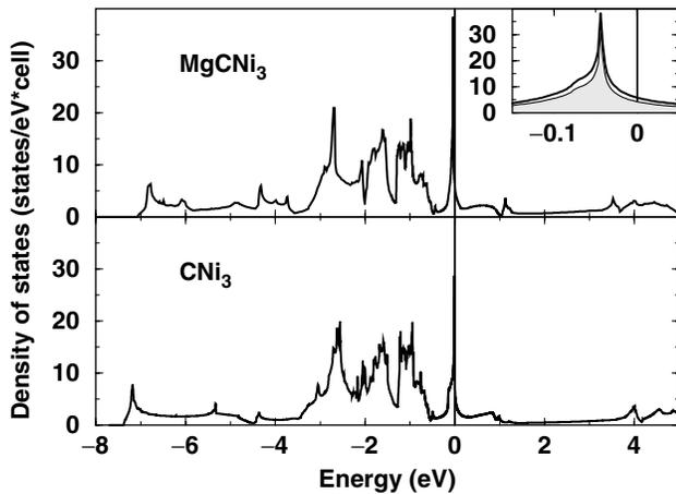
FIG. 1. The density of states of  $\text{MgCNi}_3$  (top panel), showing the nearly filled Ni  $d$  states and the extremely sharp and narrow peak just below  $E_F$  arising from a van Hove singularity. The inset gives a blowup of the peak, with the shaded portion indicating the dominant Ni  $3d$  contribution. The lower panel shows the density of states for  $\square^{2+}\text{CNi}_3$  (see text).
