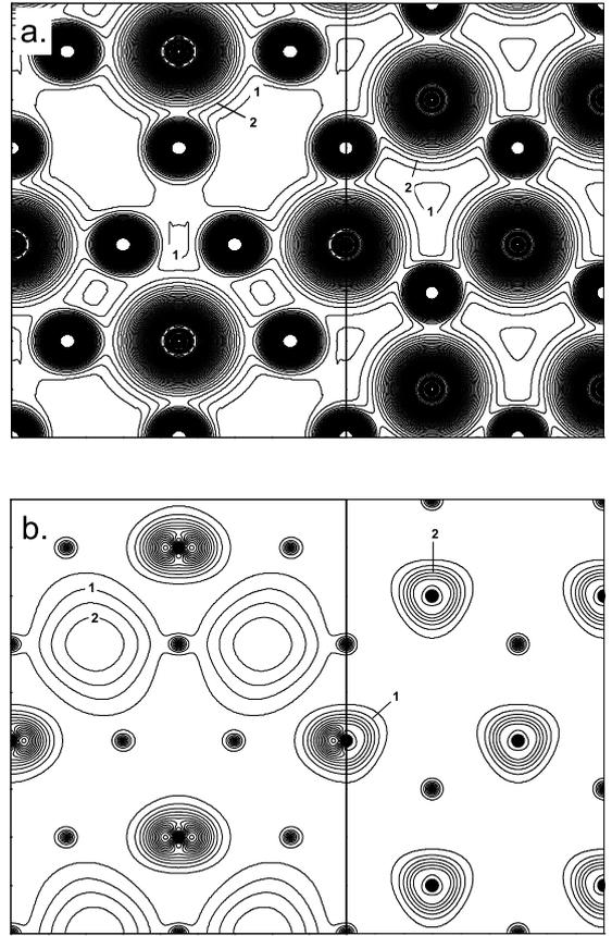
FIG. 6:  $\beta$ - $\text{Li}_3\text{N}$  valence density (a) and (unoccupied) inter-layer band density (b) contours perpendicular to the basal plane (left panels) and within the basal plane (right panels). Large regions of white space in (a) signify very low density whereas the contours in the same areas in (b) denote a maximum in the IL density. Contour lines are labeled in units of  $0.1 e/\text{\AA}^3$  and separated by  $0.05 e/\text{\AA}^3$ .
