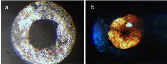
FIG. 8: (Color online) Sample image at ambient pressure (a) and at the  $\beta \rightarrow \gamma$  phase transition near 40 GPa (b). The bright spot at 40 GPa is the ruby grain used for pressure calibration.
