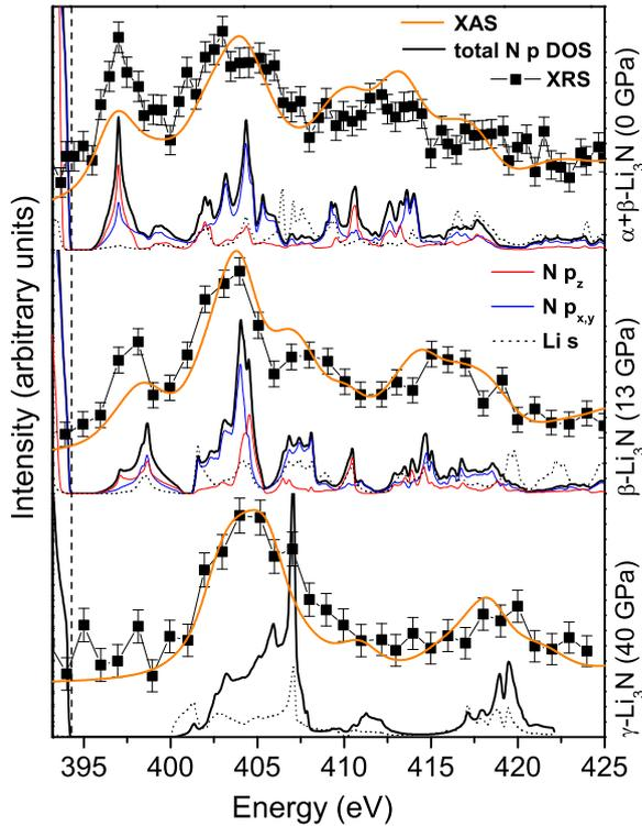
FIG. 3: (Color online) Measured nitrogen k-edge XRS spectra from the three phases of  $\text{Li}_3\text{N}$  compared with calculated Nitrogen p and Lithium s projected density of states and with the calculated X-ray absorption spectrum. The calculated curves were offset by 394.2 eV (arbitrary) in every case, for the sake of qualitative comparison with the experimental results. The vertical dashed line indicates the calculated energy of highest occupied valence states.
