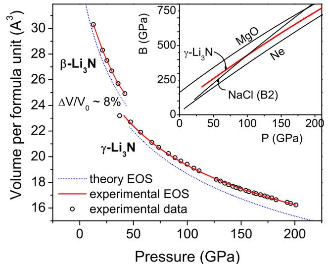
FIG. 2: (Color online) Experimental and calculated equation of state of  $\beta$ - and  $\gamma$ - $\text{Li}_3\text{N}$ . In the inset, the high pressure bulk modulus of  $\gamma$ - $\text{Li}_3\text{N}$  is compared to other common highly compressible materials. [22, 23] (NaCl, MgO and Ne Curves are interpolated up to 200 GPa).
