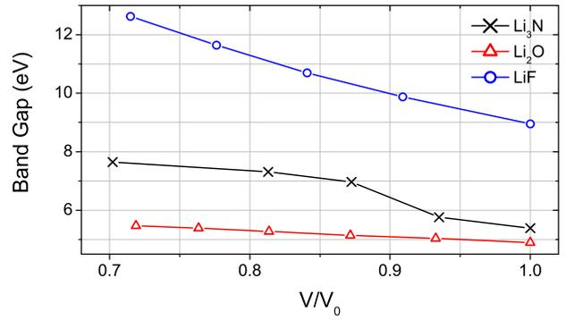
FIG. 10: Band gap increases as a function of volume reduction for related close-shelled cubic Li compounds.  $\text{LiF}$  and  $\text{Li}_2\text{O}$  are cubic at ambient pressure and  $V_0$  refers to the ambient pressure volume.  $\text{Li}_3\text{N}$   $V_0$  (in this instance alone) is taken as the volume at the  $\beta \rightarrow \gamma$  phase transition.
