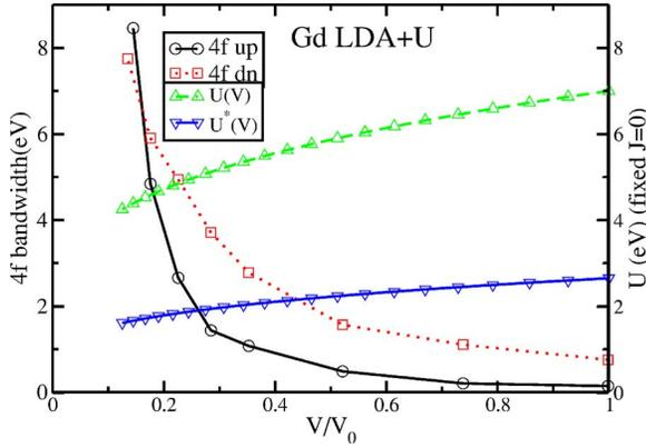
FIG. 5. (Color online) Plot of the  $4f$  bandwidths (both majority and minority), together with the volume-dependent Coulomb repulsion  $U$  from McMahan (Ref. 1). The simple crossover criterion  $W_f \approx U$  occurs around  $V/V_0 = 0.20-0.25$ , corresponding roughly to a pressure of 700–1000 GPa. Also pictured is  $U^* \equiv U/\sqrt{7}$ , see text for discussion.
