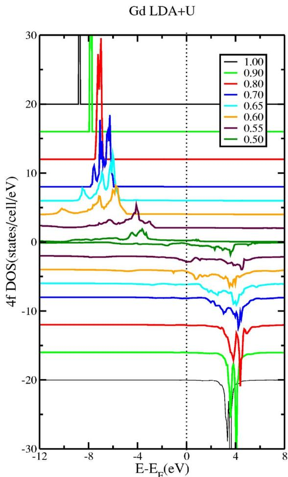
FIG. 3. (Color online) View of the  $4f$  projected density of states under compression, with majority spin plotted upward and minority spin plotted downward. The curves are displaced for clarity, by an amount proportional to the reduction in lattice constant. The legend provides the ratio  $a/a_0$ , which is decreasing from above, and from below, toward the middle of the figure.
