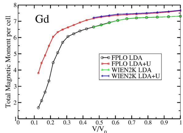
FIG. 2. (Color online) Behavior of the calculated moment per cell ( $4f$  spin moment plus conduction electron polarization) of Gd vs reduction in volume, from both LDA and LDA+U methods. For the more realistic LDA+U method, there is very little decrease in moment down to  $V/V_0=0.45$  ( $\sim 110$  GPa), with a rapid decline beginning only around  $V/V_0 \approx 0.2$  (1.5 TPa).
