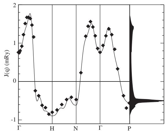
Fig. 2. The  $\mathbf{q}$ -dependent exchange constants calculated along the high symmetry lines (diamonds) and the fit obtained from values on a regular mesh throughout the Brillouin zone. Density of modes is shown in the right panel. For details see Ref. [12].
