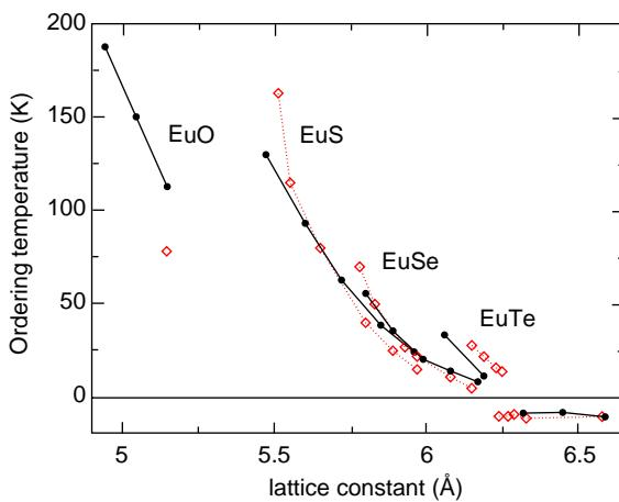
Fig. 1. The Curie and Néel (shown negative) temperatures of Eu monochalcogenides calculated with  $U = 6$  eV (full dots) compared to experimental values [10,11] (diamonds). The lines serve as guides to eyes.
