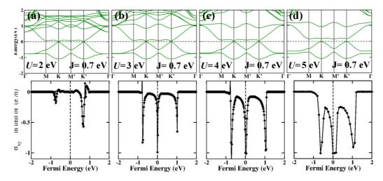
FIG. 6. Band structure (top row) and corresponding anomalous Hall conductivity in units of quantum conductance  $(e^2/h)$  (bottom row) of  $(LaMnO_3)_2/(LaAlO_3)_4$  as a function of Hubbard U in P321 symmetry. Note that the band gap at K opens above U = 3 eV, J = 0.7 eV.
