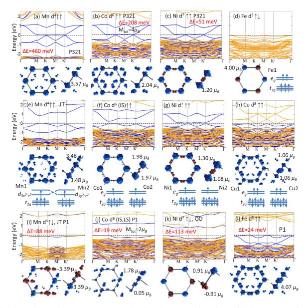
FIG. 2. Same as Fig. 1, but for  $e_g$  systems X = Mn, Fe, Co, Ni, and Cu. A common feature is a set of four bands: two nearly flat and two crossing at K and K'. Despite the formally different band filling in X = Mn, Co, Ni the Dirac points are pinned at the Fermi level within P321 symmetry (a)–(c), while symmetry breaking results in a gap opening (d)–(g). Further metastable phases are shown in (i)–(1).
