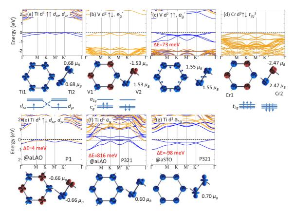
FIG. 1. Electronic ground [(a), (b), (d)] and selected metastable states [(c), (e)–(g)] in  $(LaXO_3)_2/(LaAlO_3)_4(111)$  for  $t_{2g}$  systems X = Ti, V, Cr. The majority (minority) bands are shown in blue (orange), for the isosurfaces of the spin density majority (minority) are in blue (red). In cases (a), (e)–(g), the integration range is from  $E_F$ -1 eV to  $E_F$  to emphasize the orbital polarization. Energies of metastable states are provided in red.
