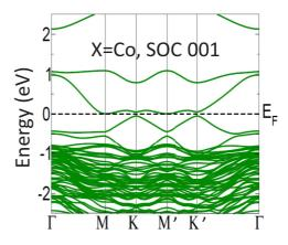
FIG. 5. Influence of SOC with magnetization axis along [001] on the band structure of  $(LaCoO_3)_2(LaAlO_3)_4(111)$  within P321 symmetry. Note the gap opening at K and the lifting of degeneracy at  $\Gamma$ .
