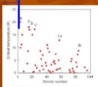
Figure 11. Highest critical temperature of simple elements as a function of the atomic number.
