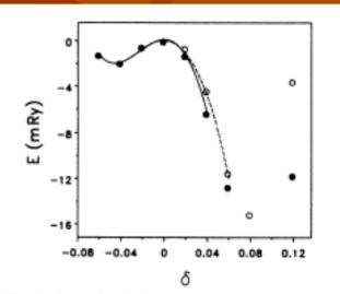
FIG. 3. The solid circles are calculated total energies for small trigonal distortions of  $B_1$ -MoN, while the open circles are for its orthorhombic distortions. The values are given relative to the energy of the  $B_1$  structure which is -8199.462.25 Ry, and the relative energies for the orthorhombic distortions have been multiplied by 3. The lines are the least-squares fit in small regions around the  $B_1$  structure.
