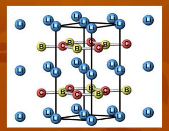
Structurally, chemically, similar to MgB<sub>2</sub> Semiconductor, so hole-doping is required (de-intercalation of Li) Deformation potential 50% larger than MgB<sub>2</sub>  $T_c = 75$  K might be realistic estimate
